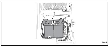
Figure 4-22 Battery and Connections
